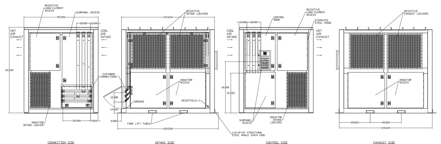
CONNECTION SIDE INTAKE SIDE CONTROL SIDE -129,250 4.000 I<del>---|-4</del>.000 **-**0.562 NOTES: ADD HOLE PATTERN AS REQUIRED 1. CONSTRUCTION: ALL WELDED FORMED STEEL FRAME, DOORS, PANELS AND SKID. 1/2" THICK FLANGE
