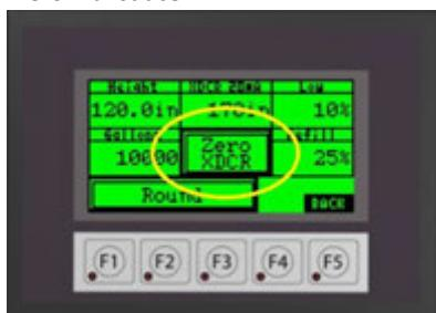
Once the tank shape, height and volume have been set, the level transducer for the tank must be calibrated (zeroed). To do so, remove the probe from the tank or hold it above the fluid level and press and release the "Zero XDCR" button several times to ensure the measurement is accurate. When finished, install/return the probe to the tank. (See *Zero Transducer*)
