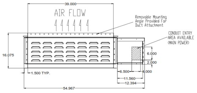
Example of a Simplex Vector Duct Mounted Load Bank
