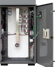
The load bank enclosure is of double wall construction for cool exterior and thermal isolation of the load elements. Cooling airflow through the enclosure is vertical with cold air intake at the bottom and hot air exhaust out the top. Intake and exhaust openings are screened. Enclosure is powder-coated dark gray. Hood powder-coated high temperature black.
