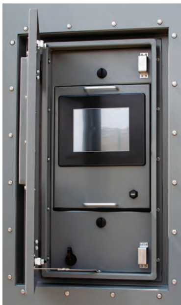
The touchscreen operator interface mounted in a protective enclosure is removable for remote control.
