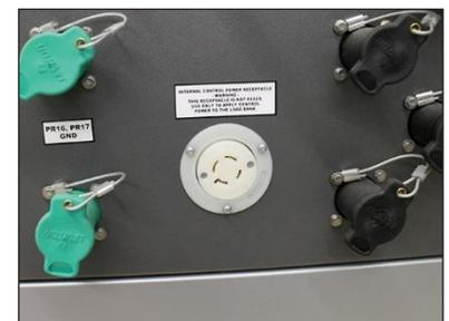
and fan power, plug the Fan/Control Power Plug into the receptacle on the back of the load bank (see **Figure 3 on page 13**). If you will be using external power, plug the Control Power Plug into a 230/460V, 3-phase, 60Hz, 20A receptacle.
