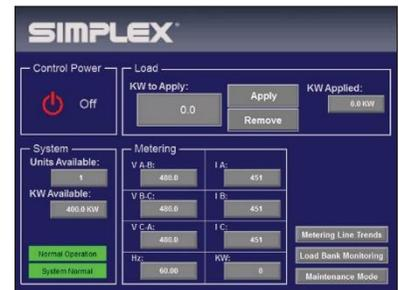
**Figure 9: Single Unit Monitoring Screen**
