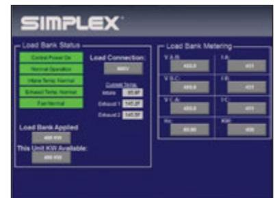
If you want to record this data, insert a USB drive into the port below the screen and press the “Data Logging Disabled” button. When you are done, press the button again and the load bank will write the data in a tab-delimited format to the thumb drive.
