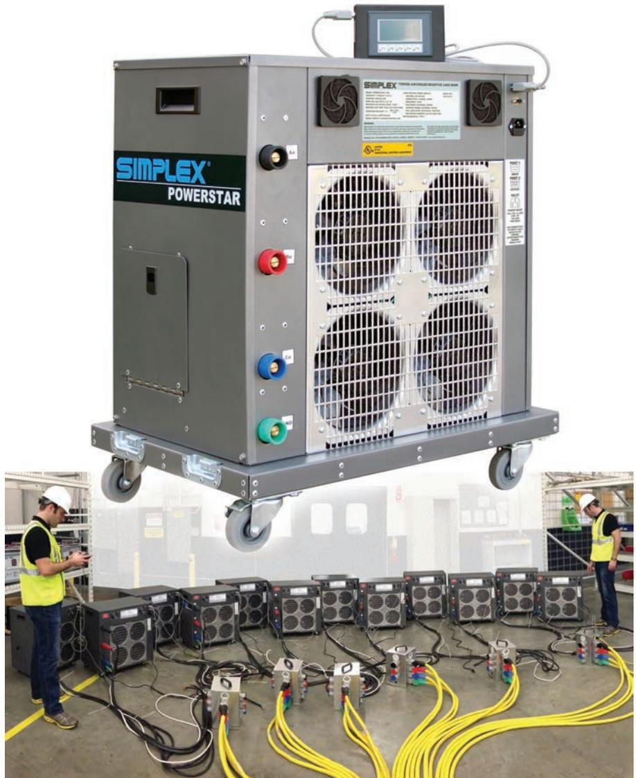
Parallel and network up to 40 Powerstar Load Banks with control and data acquisition from a single controller. When networked, load is proportioned equally across all load banks. System automatically sequesters failed unit.
